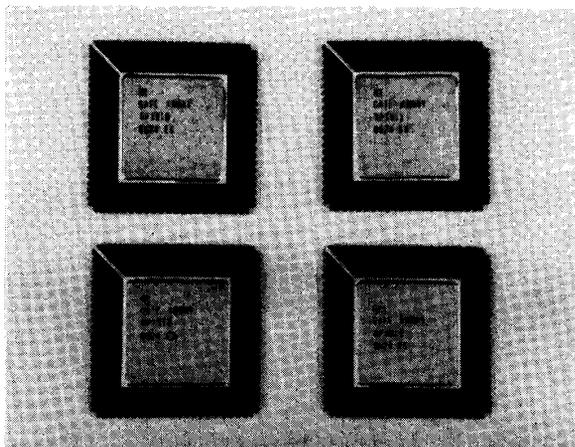
Fig. 7. Four 3  $\mu\text{m}$  CMOS chips fabricated by GE to verify the 2-D FFT design. These include the memory crossbar switch, adder/subtractor, and partitioned multiplier chips.
