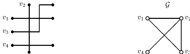
Figure 1: Routing of 4 nets and graph G representing all potential short faults between nets.
