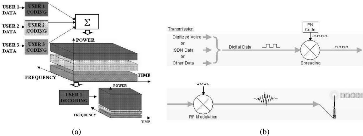
Fig. 1. (a) Demonstration of code-division multiplexing (b) Transmitter structure of a CDMA system.
