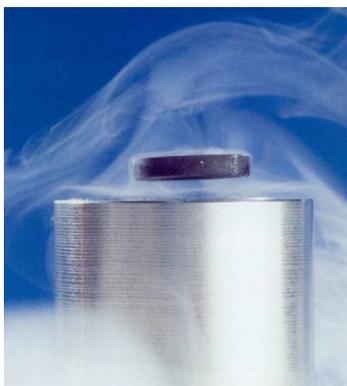
Figure 1: Superconductors levitate because magnetic fields bend around them (courtesy of Argonne)
