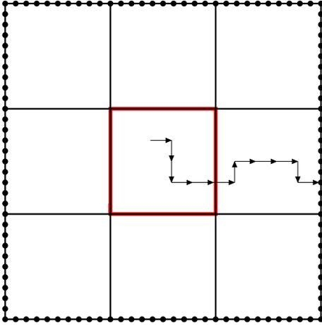
**Fig. 3. The proof of the lower bounds in Theorem 4.** Black dots represent the root on the boundary of  $[3n]^d$  for each component of the spanning forest. The red square highlights the central subcube; the water from this subcube must travel to a root on the boundary, and to do so it must first cross its own boundary, and then pass through at least  $n$  additional vertices.
